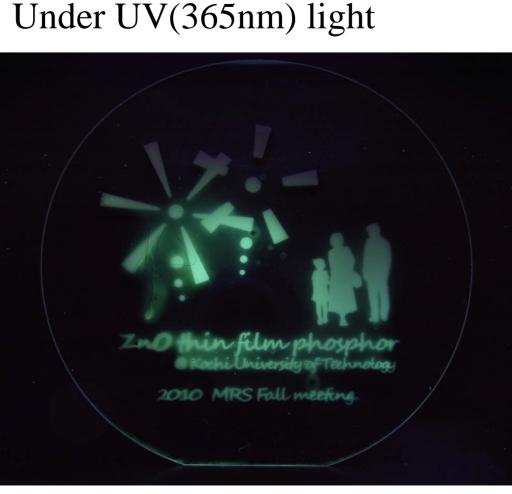
Precisely patterned ZnO thin film phosphor was achieved successfully after low temperature post-treatment. Ref 2: C. Li et al.: patent application, 2011-7387 (2011.1.17)
